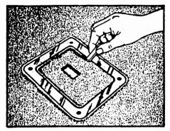
Remove the boot and place the chrome plated retainer plate exactly within the scribed outline.Scribe the inside opening of the plate on the carpet with chalk.
