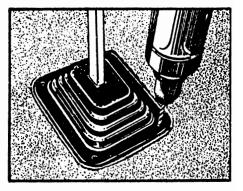
4. Replace the boot.Drill 1/8" diam. holes through floor using boot holes to locate hole positions.
