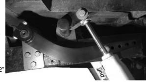
Note: You can weld this assembly onto the frame but just remember you will have to grind off the welds if you ever need to remove the torsion bar. Just be sure to check the back side for any fuel or brake lines that could be damaged.
