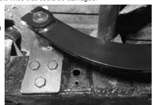
½" Nyloc Nuts to secure the truss bracket. Once you have the truss bracket attached to the truss tighten all the hardware and bolt the shock back into place.
