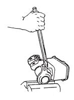
Clamp master cylinder in vise as shown. Insert prybar and lift up on end with a slow firm pressure until reservoir pulls away from the rubber seals.
