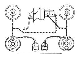
Due to the split system it is sometimes necessary to leave one bleeder screw open in the front if rear wheels are bled and vice versa. Always use bleeder screw and jar as shown to avoid air being sucked back into system.
