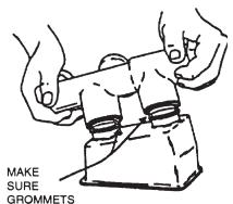
ARE IN PLACE AND RESERVOIR IS COMPLETELY INSERTED. LUBRICATE RUBBER GROMMETS WITH BRAKE FLUID.
