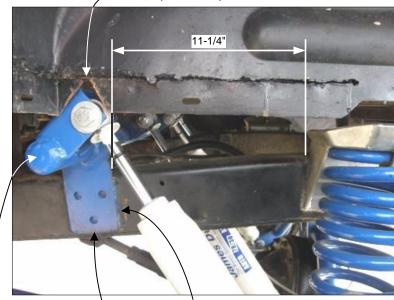
Mount could be welded instead of bolted onto frame
