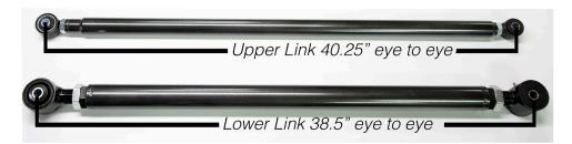
Thread the LH 1.25"-12 Jam Nuts onto the 1 1/4-12 DDB Ends. Then thread the DDB ends into the Left Hand end of the lower link bars. The left hand side is distinguished by a groove on the end of the link. Do not tighten all the way. Repeat these steps for the Right Hand side using the Large Poly Ends. Using a tape measure make sure the bar is 38.5" inches from center of LH to RH mounting point (eye to eye).
