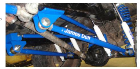
Thread the LH 3/4"-16 Jam Nuts onto the 3/4-16 DDB Ends. Then thread the DDB ends into the Left Hand end of the upper link bars. The left hand side is distinguished by a groove on the end of the link. Do not tighten all the way. Repeat these steps for the Right Hand side using the small Poly Ends. Using a tape measure make sure the bar is 40.25" inches from center of LH to RH mounting point (eye to eye).
