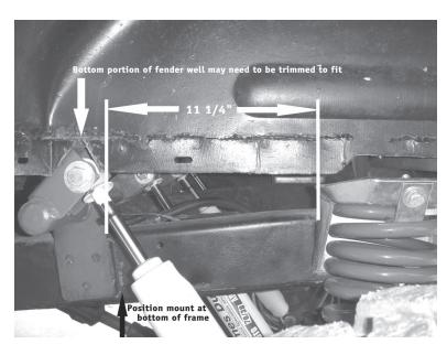
Note: position the mount at the bottom of frame as shown. Note: Mount can be welded instead of bolted onto frame.
