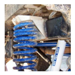
Note: The coil towers' placement on the frame will vary based on the ride height or overall lift size of your vehicle, as well as the weight of the vehicle and its compression on the springs. Once ideal height placement is achieved and the springs are vertically aligned, we suggest to 'Tack weld' coil towers in place on both frame rails. We say 'Tack weld' so the towers are secure but not over welded in the event of misalignment and need to reposition either side.
